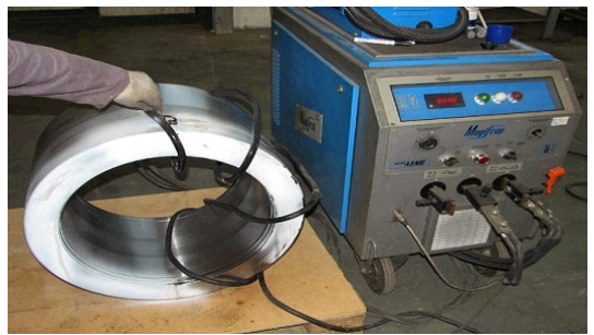
MAGNETIC PARTICLE INSPECTION
