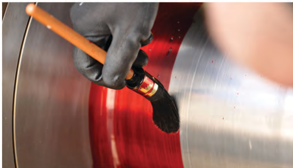
Dye Penetrant Testing
