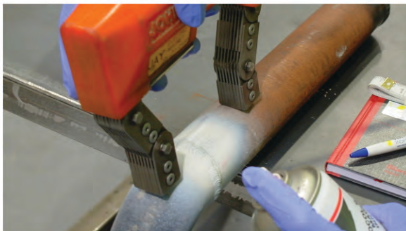
Magnetic Particle Inspection
