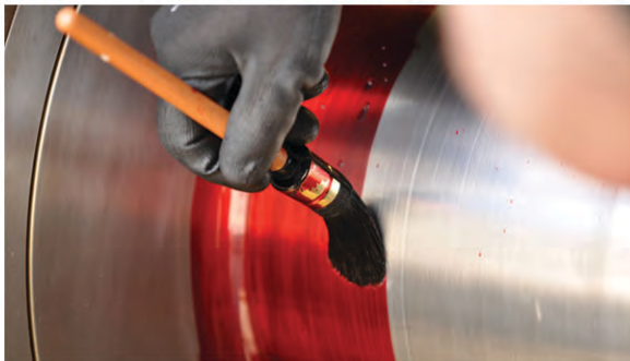
Dye Penetrant Testing
